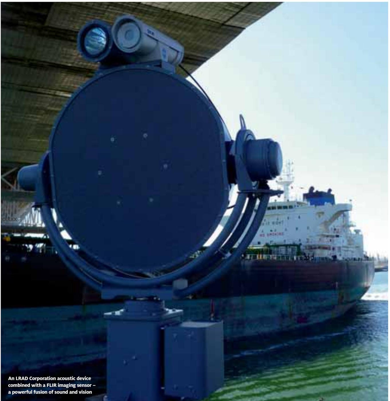
An LRAD Corporation acoustic device combined with a FLIR imaging sensor – a powerful fusion of sound and vision
