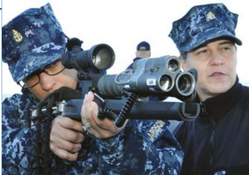
BE Meyers' Glare LA-9/P green laser can deliver warnings out to 4km at night and 1.5km in daylight. (Photo: USN)
